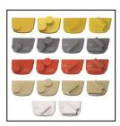
**QuickChange System and Tooling** feature extremely fast and convenient tool changes, and a long tool life, providing for great long-term cost savings. The QuickChange pads are produced in four different bonds for super hard, hard, medium and soft concrete, in a variety of grit sizes. They are offered with 1 or 2 buttons or rectangular segments, which allows you to customize the aggressiveness of the cut.
